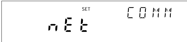
Communications display for setting the network type
